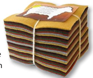
*Felt is a nonwoven material produced by matting, condensing, and pressing fibers together.*
