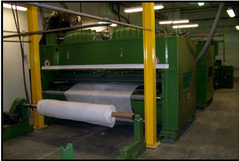
National Nonwovens' newly installed 2.4 meter air-laid needlepunch nonwoven line can produce products in the range 1.5 oz/yd<sup>2</sup> to 10 oz/yd<sup>2</sup>, supported or unsupported. It is strategically located in a contained, clean-room environment. Total processing capacity on this line is in excess of 2 million pounds of fiber per year.
